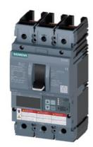
Circuit breaker 3VA6 UL frame 250 breaking capacity class C 100kA @ 480V 3-pole, Line protection ETU830, LIG, In=250A overload protection, 100% rated Ir=100A...250A Short-circuit protection Ii=1.5...10 x In Ground-fault protection Ig=0.2...1 x In, tg=0.05-0.8s without connection
