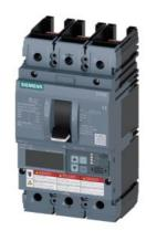
circuit breaker 3VA6 UL frame 250 breaking capacity class C 100kA @ 480V 3-pole, line protection ETU830, LIG, In=250A overload protection Ir=100A...250A short-circuit protection Ii=1.5...10 x In ground-fault protection Ig=0.2...1 x In, tg=0.05-0.8s without connection
