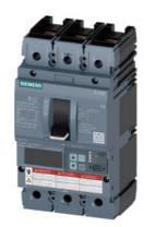
Circuit breaker 3VA6 UL frame 250 breaking capacity class C 100kA @ 480 V 3pole, Line protection ETU556, LSI, In=250A overload protection, 100% rated Ir=100A ...250A Short-circuit protection Isd=0.6..10x In, Ii=1.5..10x In N conductor protection optionally with external CT; up to 160% Ground-fault alarm message via EFB300 or COM nut keeper kit on both sides
