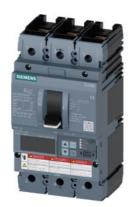
Circuit breaker 3VA6 UL frame 250 breaking capacity class C 100kA @ 480 V 3-pole, Line protection ETU560, LSIG, In=250A overload protection, 100% rated Ir=100A ...250A Short-circuit protection Isd=0.6..10x In, Ii=1.5..10x In N conductor protection optionally with external CT; up to 160% Ground-fault protection Ig=0.2... 1 x In, tg=0.05-0.8s nut keeper kit on both sides
