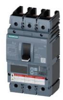
Circuit breaker 3VA6 UL frame 250 breaking capacity class C 100kA @ 480V 3pole, Line protection ETU560, LSIG, In=250A overload protection, 100% rated Ir=100A...250A Short-circuit protection Isd=0.6..10x In, Ii=1.5..10x In N conductor protection optionally with external CT, up to 160% Ground-fault protection Ig=0.2...1 x In, tg=0.05-0.8s without connection
