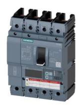
Circuit breaker 3VA6 UL frame 250 breaking capacity class C 100kA @ 480V 4-pole, Line protection ETU550, LSI, In=250A overload protection, 100% rated Ir=100A...250A Short-circuit protection Isd=0.6..10x In, Ii=1.5..10x In N conductor protection adjustable (OFF, up to 100%) without connection
