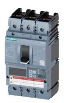
Circuit breaker 3VA6 UL frame 250 breaking capacity class H 65kA @ 480 V 3-pole, Line protection ETU856, LSI, In=250A overload protection, 100% rated Ir=100A ...250A Short-circuit protection Isd=0.6..10x In, Ii=1.5..10x In N conductor protection optionally with external CT; up to 160% Ground-fault alarm message via EFB300 or COM cable connection on both sides
