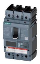
Circuit breaker 3VA6 UL frame 250 breaking capacity class H 65kA @ 480 V 3-pole, Line protection ETU856, LSI, In=250A overload protection, 100% rated Ir=100A ...250A Short-circuit protection Isd=0.6..10x In, Ii=1.5..10x In N conductor protection optionally with external CT; up to 160% Ground-fault alarm message via EFB300 or COM nut keeper kit on both sides
