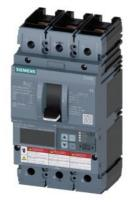
circuit breaker 3VA6 UL frame 250 breaking capacity class H 65kA @ 480 V 3-pole, line protection ETU856, LSI, In=250A overload protection Ir=100A ...250A short-circuit protection Isd=0.6..10x In, Ii=1.5..10x In N conductor protection opt. w. ext. CT; up to 160% ground-fault alarm message via EFB300 or COM nut keeper kit on both sides
