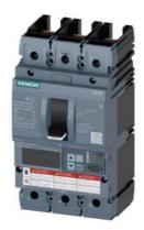
Circuit breaker 3VA6 UL frame 250 breaking capacity class H 65kA @ 480V 3-pole, Line protection ETU856, LSI, In=250A overload protection, 100% rated Ir=100A...250A Short-circuit protection Isd=0.6..10x In, Ii=1.5..10x In N conductor protection optionally with external CT, up to 160% Ground-fault alarm message via EFB300 or COM without connection
