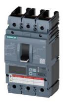
circuit breaker 3VA6 UL frame 250 breaking capacity class H 65kA @ 480V 3-pole, line protection ETU856, LSI, In=250A overload protection Ir=100A...250A short-circuit protection Isd=0.6..10x In, Ii=1.5..10x In N conductor protection optionally with external current transformer, up to 160% ground-fault alarm message via EFB300 or COM without connection
