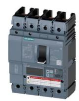
Circuit breaker 3VA6 UL frame 250 breaking capacity class H 65kA @ 480V 4pole, Line protection ETU860, LSIG, In=250A overload protection, 100% rated Ir=100A...250A Short-circuit protection Isd=0.6..10x In, Ii=1.5..10x In N conductor protection adjustable (OFF, up to 100%) Ground-fault protection Ig=0.2...1 x In= tg=0.05-0.8s without connection
