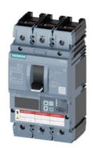
Circuit breaker 3VA6 UL frame 250 breaking capacity class H 65kA @ 480 V 3-pole, Line protection ETU860, LSIG, In=250A overload protection, 100% rated Ir=100A ...250A Short-circuit protection Isd=0.6..10x In, Ii=1.5..10x In N conductor protection optionally with external CT; up to 160% Ground-fault protection Ig=0.2... 1 x In, tg=0.05-0.8s cable connection on both sides
