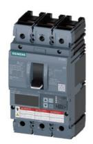
circuit breaker 3VA6 UL frame 250 breaking capacity class H 65kA @ 480 V 3-pole, line protection ETU860, LSIG, In=250A overload protection Ir=100A ...250A short-circuit protection Isd=0.6..10x In, Ii=1.5..10x In N conductor protection opt. w. ext. CT; up to 160% ground-fault protection Ig=0.2... 1 x In, tg=0.05-0.8s nut keeper kit on both sides
