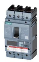
Circuit breaker 3VA6 UL frame 250 breaking capacity class H 65kA @ 480 V 3-pole, Line protection ETU850, LSI, In=250A overload protection, 100% rated Ir=100A ...250A Short-circuit protection Isd=0.6..10x In, Ii=1.5..10x In N conductor protection optionally with external CT; up to 160% cable connection on both sides
