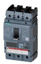
Circuit breaker 3VA6 UL frame 250 breaking capacity class H 65kA @ 480 V 3-pole, Line protection ETU850, LSI, In=250A overload protection, 100% rated Ir=100A ...250A Short-circuit protection Isd=0.6..10x In, Ii=1.5..10x In N conductor protection optionally with external CT; up to 160% nut keeper kit on both sides
