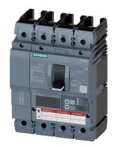
Circuit breaker 3VA6 UL frame 250 breaking capacity class H 65kA @ 480V 4-pole, Line protection ETU830, LIG, In=250A overload protection, 100% rated Ir=100A...250A Short-circuit protection Ii=1.5...10 x In Ground-fault protection Ig=0.2...1 x In, tg=0.05-0.8s without connection
