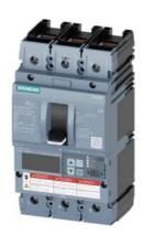
Circuit breaker 3VA6 UL frame 250 breaking capacity class H 65kA @ 480 V 3-pole, Line protection ETU830, LIG, In=250A overload protection, 100% rated Ir=100A ...250A Short-circuit protection Ii=1.5...10 x In Ground-fault protection Ig=0.2... 1 x In, tg=0.05-0.8s cable connection on both sides
