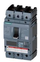
Circuit breaker 3VA6 UL frame 250 breaking capacity class H 65kA @ 480 V 3-pole, Line protection ETU830, LIG, In=250A overload protection, 100% rated Ir=100A ...250A Short-circuit protection Ii=1.5...10 x In Ground-fault protection Ig=0.2... 1 x In, tg=0.05-0.8s nut keeper kit on both sides
