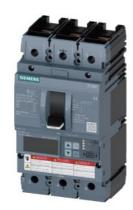
circuit breaker 3VA6 UL frame 250 breaking capacity class H 65kA @ 480 V 3-pole, line protection ETU830, LIG, In=250A overload protection Ir=100A ...250A short-circuit protection Ii=1.5...10 x In ground-fault protection Ig=0.2... 1 x In, tg=0.05-0.8s nut keeper kit on both sides
