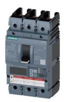
Circuit breaker 3VA6 UL frame 250 breaking capacity class H 65kA @ 480V 3-pole, Line protection ETU830, LIG, In=250A overload protection, 100% rated Ir=100A...250A Short-circuit protection Ii=1.5...10 x In Ground-fault protection Ig=0.2...1 x In, tg=0.05-0.8s without connection
