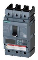
circuit breaker 3VA6 UL frame 250 breaking capacity class H 65kA @ 480V 3-pole, line protection ETU830, LIG, In=250A overload protection Ir=100A...250A short-circuit protection Ii=1.5...10 x In ground-fault protection Ig=0.2...1 x In, tg=0.05-0.8s without connection
