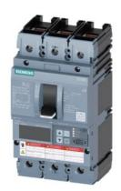
Circuit breaker 3VA6 UL frame 250 breaking capacity class H 65kA @ 480 V 3-pole, Line protection ETU820, LI, In=250A overload protection, 100% rated Ir=100A ...250A Short-circuit protection Ii=1.5...10 x In cable connection on both sides
