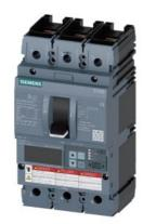
Circuit breaker 3VA6 UL frame 250 breaking capacity class H 65kA @ 480 V 3pole, Line protection ETU820, LI, In=250A overload protection, 100% rated Ir=100A ...250A Short-circuit protection Ii=1.5...10 x In nut keeper kit on both sides
