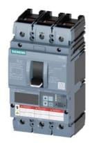
Circuit breaker 3VA6 UL frame 250 breaking capacity class H 65kA @ 480 V 3-pole, Line protection ETU556, LSI, In=250A overload protection, 100% rated Ir=100A ...250A Short-circuit protection Isd=0.6..10x In, Ii=1.5..10x In N conductor protection optionally with external CT; up to 160% Ground-fault alarm message via EFB300 or COM cable connection on both sides
