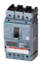
circuit breaker 3VA6 UL frame 250 breaking capacity class H 65kA @ 480 V 3-pole, line protection ETU556, LSI, In=250A overload protection Ir=100A ...250A short-circuit protection Isd=0.6..10x In, Ii=1.5..10x In N conductor protection opt. w. ext. CT; up to 160% ground-fault alarm message via EFB300 or COM cable connection on both sides
