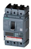
Circuit breaker 3VA6 UL frame 250 breaking capacity class H 65kA @ 480 V 3pole, Line protection ETU556, LSI, In=250A overload protection, 100% rated Ir=100A ...250A Short-circuit protection Isd=0.6..10x In, Ii=1.5..10x In N conductor protection optionally with external CT; up to 160% Ground-fault alarm message via EFB300 or COM nut keeper kit on both sides
