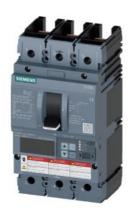
Circuit breaker 3VA6 UL frame 250 breaking capacity class H 65kA @ 480V 3-pole, Line protection ETU556, LSI, In=250A overload protection, 100% rated Ir=100A...250A Short-circuit protection Isd=0.6..10x In, Ii=1.5..10x In N conductor protection optionally with external CT, up to 160% Ground-fault alarm message via EFB300 or COM without connection
