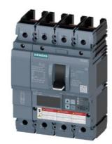
Circuit breaker 3VA6 UL frame 250 breaking capacity class H 65kA @ 480V 4pole, Line protection ETU560, LSIG, In=250A overload protection, 100% rated Ir=100A...250A Short-circuit protection Isd=0.6..10x In, Ii=1.5..10x In N conductor protection adjustable (OFF, up to 100%) Ground-fault protection Ig=0.2...1 x In= tg=0.05-0.8s without connection
