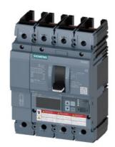
circuit breaker 3VA6 UL frame 250 breaking capacity class H 65kA @ 480V 4-pole, line protection ETU560, LSIG, In=250A overload protection Ir=100A...250A short-circuit protection Isd=0.6..10x In, Ii=1.5..10x In N conductor protection adjustable (OFF, up to 100%) ground-fault protection Ig=0.2...1 x In= tg=0.05-0.8s without connection
