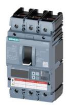
Circuit breaker 3VA6 UL frame 250 breaking capacity class H 65kA @ 480 V 3-pole, Line protection ETU560, LSIG, In=250A overload protection, 100% rated Ir=100A ...250A Short-circuit protection Isd=0.6..10x In, Ii=1.5..10x In N conductor protection optionally with external CT; up to 160% Ground-fault protection Ig=0.2... 1 x In, tg=0.05-0.8s cable connection on both sides
