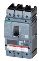
circuit breaker 3VA6 UL frame 250 breaking capacity class H 65kA @ 480 V 3-pole, line protection ETU560, LSIG, In=250A overload protection Ir=100A ...250A short-circuit protection Isd=0.6..10x In, Ii=1.5..10x In N conductor protection opt. w. ext. CT; up to 160% ground-fault protection Ig=0.2... 1 x In, tg=0.05-0.8s cable connection on both sides
