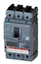
circuit breaker 3VA6 UL frame 250 breaking capacity class H 65kA @ 480 V 3-pole, line protection ETU560, LSIG, In=250A overload protection Ir=100A ...250A short-circuit protection Isd=0.6..10x In, Ii=1.5..10x In N conductor protection opt. w. ext. CT; up to 160% ground-fault protection Ig=0.2... 1 x In, tg=0.05-0.8s nut keeper kit on both sides
