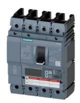
Circuit breaker 3VA6 UL frame 250 breaking capacity class H 65kA @ 480V 4-pole, Line protection ETU550, LSI, In=250A overload protection, 100% rated Ir=100A...250A Short-circuit protection Isd=0.6..10x In, Ii=1.5..10x In N conductor protection adjustable (OFF, up to 100%) without connection
