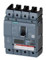
circuit breaker 3VA6 UL frame 250 breaking capacity class H 65kA @ 480V 4-pole, line protection ETU550, LSI, In=250A overload protection Ir=100A...250A short-circuit protection Isd=0.6..10x In, Ii=1.5..10x In N conductor protection adjustable (OFF, up to 100%) without connection
