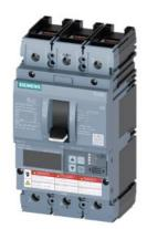
Circuit breaker 3VA6 UL frame 250 breaking capacity class H 65kA @ 480 V 3-pole, Line protection ETU550, LSI, In=250A overload protection, 100% rated Ir=100A ...250A Short-circuit protection Isd=0.6..10x In, Ii=1.5..10x In N conductor protection optionally with external CT; up to 160% cable connection on both sides
