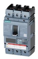
circuit breaker 3VA6 UL frame 250 breaking capacity class H 65kA @ 480 V 3-pole, line protection ETU550, LSI, ln=250A overload protection lr=100A ...250A short-circuit protection lsd=0.6..10x ln, li=1.5..10x ln N conductor protection opt. w. ext. CT; up to 160% cable connection on both sides
