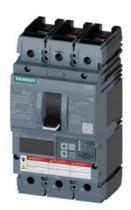
Circuit breaker 3VA6 UL frame 250 breaking capacity class H 65kA @ 480 V 3-pole, Line protection ETU550, LSI, In=250A overload protection, 100% rated Ir=100A ...250A Short-circuit protection Isd=0.6..10x In, Ii=1.5..10x In N conductor protection optionally with external CT; up to 160% nut keeper kit on both sides
