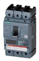
circuit breaker 3VA6 UL frame 250 breaking capacity class H 65kA @ 480 V 3-pole, line protection ETU550, LSI, In=250A overload protection Ir=100A ...250A short-circuit protection Isd=0.6..10x In, Ii=1.5..10x In N conductor protection opt. w. ext. CT; up to 160% nut keeper kit on both sides
