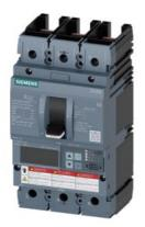
Circuit breaker 3VA6 UL frame 250 breaking capacity class H 65kA @ 480V 3-pole, Line protection ETU550, LSI, In=250A overload protection, 100% rated Ir=100A...250A Short-circuit protection Isd=0.6..10x In, Ii=1.5..10x In N conductor protection optionally with external CT, up to 160% without connection
