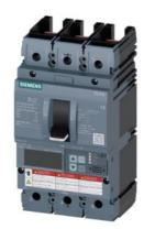
circuit breaker 3VA6 UL frame 250 breaking capacity class H 65kA @ 480V 3-pole, line protection ETU550, LSI, In=250A overload protection Ir=100A...250A short-circuit protection Isd=0.6..10x In, Ii=1.5..10x In N conductor protection optionally with external current transformer, up to 160% without connection
