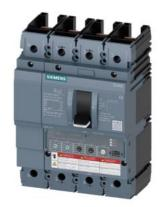
Circuit breaker 3VA6 UL frame 250 breaking capacity class H 65kA @ 480V 4-pole, Line protection ETU350, LSI, In=250A overload protection, 100% rated Ir=100A...250A Short-circuit protection Isd=1.5...10 x Ir, Ii=10 x In N conductor protection adjustable (OFF, 50%, 100%) without connection
