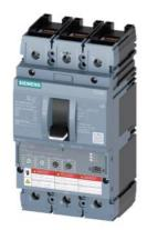
circuit breaker 3VA6 UL frame 250 breaking capacity class H 65kA @ 480 V 3-pole, line protection ETU350, LSI, In=250A overload protection Ir=100A ...250A short-circuit protection Isd=1.5... 10 x Ir, li=10 x In cable connection on both sides
