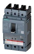
Circuit breaker 3VA6 UL frame 250 breaking capacity class H 65kA @ 480V 3-pole, Line protection ETU350, LSI, In=250A overload protection, 100% rated Ir=100A...250A Short-circuit protection Isd=1.5...10 x Ir, Ii=10 x In without connection
