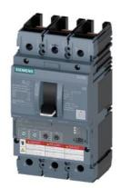
circuit breaker 3VA6 UL frame 250 breaking capacity class H 65kA @ 480V 3-pole, line protection ETU350, LSI, In=250A overload protection Ir=100A...250A short-circuit protection Isd=1.5...10 x Ir, Ii=10 x In without connection
