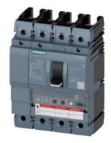
Circuit breaker 3VA6 UL frame 250 breaking capacity class H 65kA @ 480V 4-pole, Line protection ETU330, LIG, In=250A overload protection, 100% rated Ir=100A...250A Short-circuit protection Ii=1.5...10 x In N conductor protection adjustable (OFF, 50%, 100%) Ground-fault protection Ig=0.2...1 x In= tg=0.1/0.3s without connection
