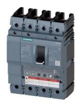
circuit breaker 3VA6 UL frame 250 breaking capacity class H 65kA @ 480V 4-pole, line protection ETU330, LIG, In=250A overload protection Ir=100A...250A short-circuit protection Ii=1.5...10 x In N conductor protection adjustable (OFF, 50%, 100%) ground-fault protection Ig=0.2...1 x In= tg=0.1/0.3s without connection
