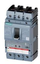
circuit breaker 3VA6 UL frame 250 breaking capacity class H 65kA @ 480 V 3-pole, line protection ETU330, LIG, In=250A overload protection Ir=100A ...250A short-circuit protection Ii=1.5...10 x In ground-fault protection Ig=0.2... 1 x In, tg=0.1/0.3s cable connection on both sides
