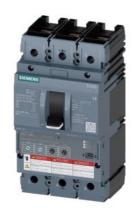
circuit breaker 3VA6 UL frame 250 breaking capacity class H 65kA @ 480 V 3-pole, line protection ETU330, LIG, In=250A overload protection Ir=100A ...250A short-circuit protection Ii=1.5...10 x In ground-fault protection Ig=0.2... 1 x In, tg=0.1/0.3s nut keeper kit on both sides
