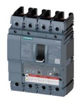
Circuit breaker 3VA6 UL frame 250 breaking capacity class H 65kA @ 480V 4-pole, Line protection ETU320, Ll, In=250A overload protection, 100% rated Ir=100A...250A Short-circuit protection Ii=1.5...10 x In N conductor protection adjustable (OFF, 50%, 100%) without connection
